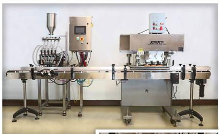
The GPM 5-Up Bellows and Piston Bottle Filling System is designed to accommodate bottle filling of liquids and viscous products on one system, without having to change controls. This is achieved by providing a system that can use a GPM 5-Up Bellows Filler for liquid and semiviscous products, or a GPM 5-Up Piston Filler for viscous products, all
